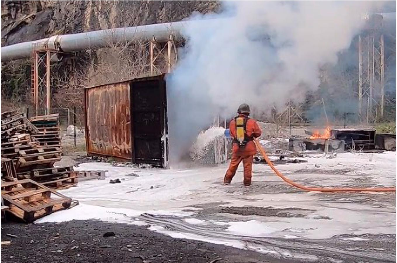
Figure 59: Using foam of a 40kWh battery fire.
