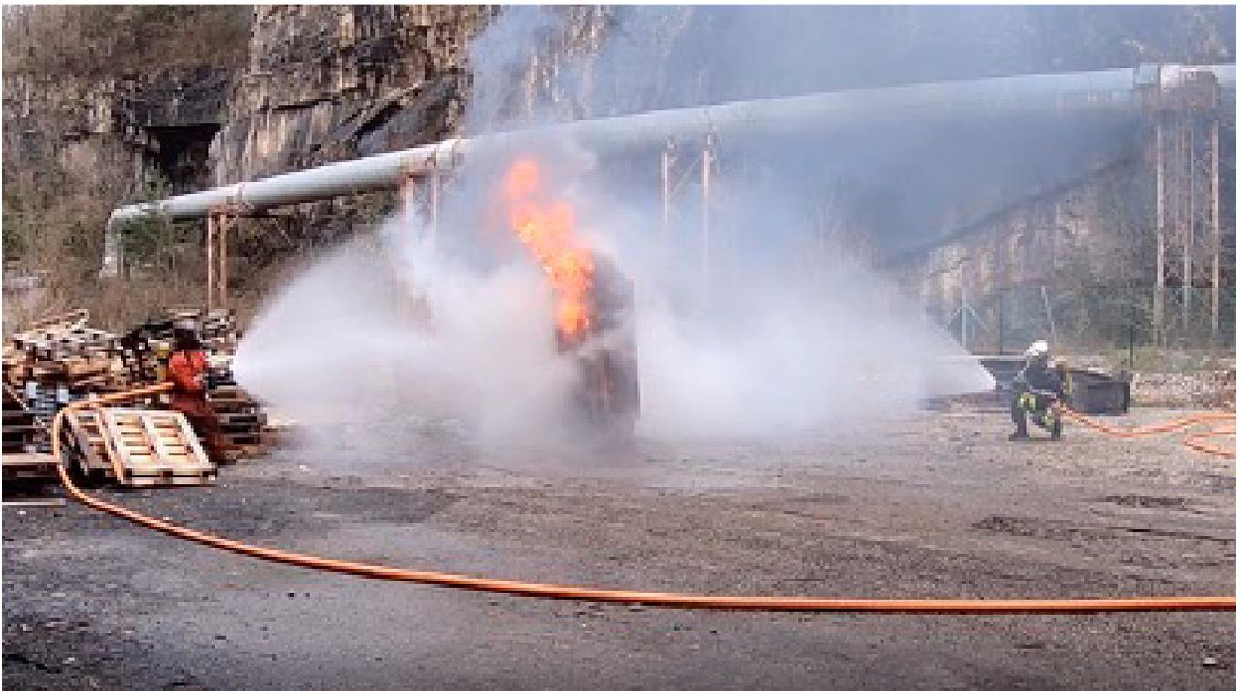
Figure 57: Using two variable flow hoses at 500L/min each on a 40kWh battery cabinet.
