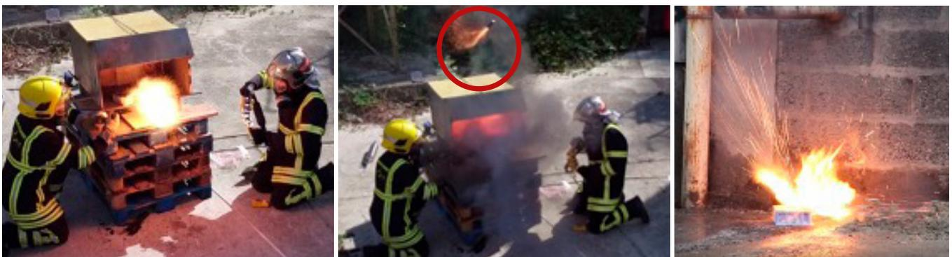
Figure 52: Projection of solid metal elements observed when burning a 30Wh storage system.
