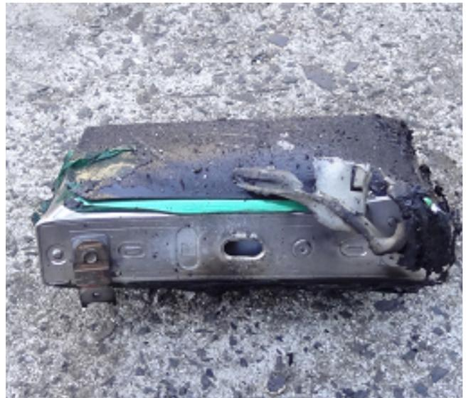
On the photos above, we can clearly see that although under pressure increase inside the cell, their casing has deformed. Also, on the module photos, we can clearly see that the casing has not withstood the heat and pressure increase of each cell and has completely opening leaving the cells to split away from each other,
