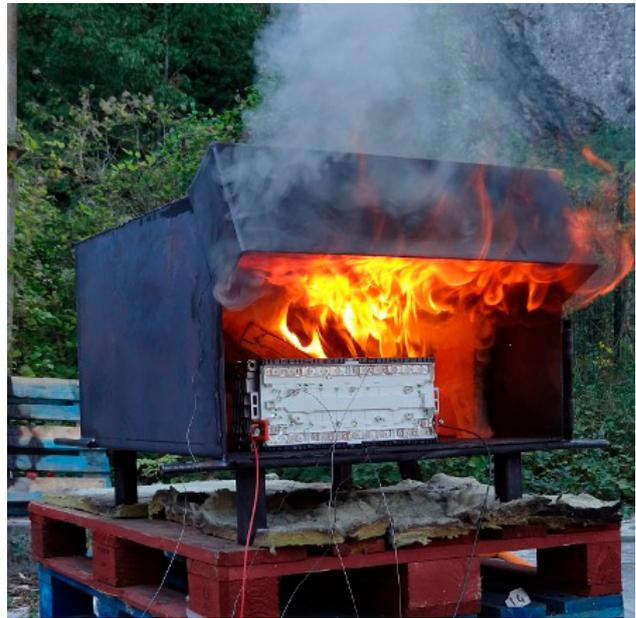
Figure 44: Photo of the module during the thermal attack test.
