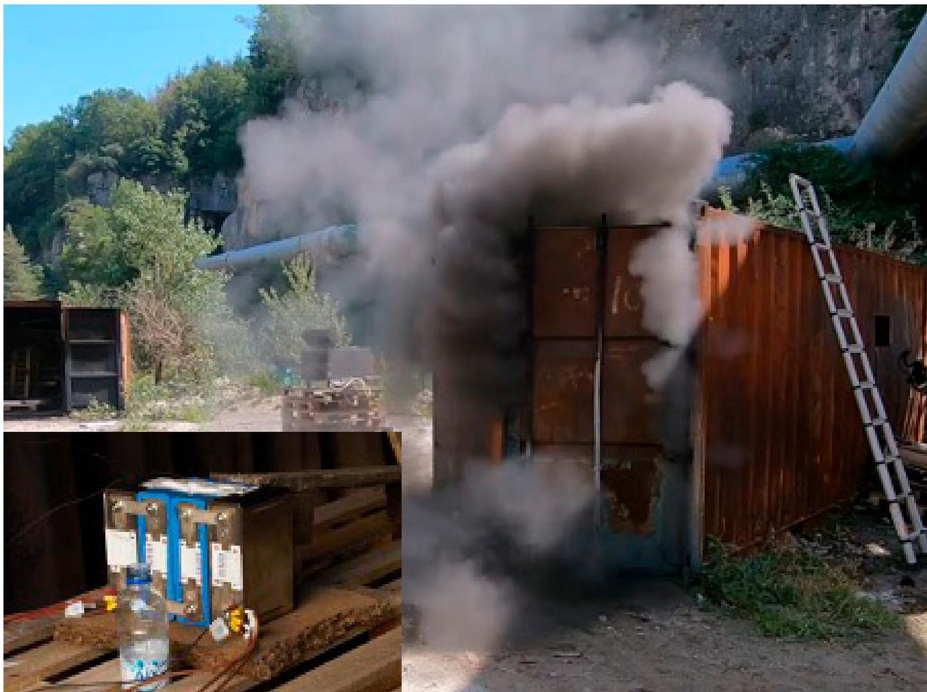
Figure 54: Explosion of fumes during an overload of a 4-cell LEV75 in a 6m shipping container.
